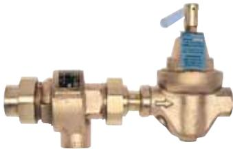
Positive protection against backflow when supply pressure falls below system pressure. Assembly combines FWR feedwater regulator and DCAP dual check assembly backflow preventer.
