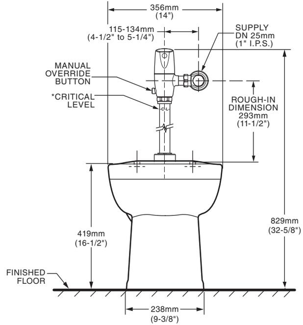
\*Note: The Critical Line (-C-L-) on Vacuum Breaker must typically be a minimum of 6" (152mm) above fixture. Consult Codes for details.
