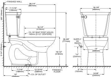
THIS TOILET IS DESIGNED TO ROUGH-IN AT A MINIMUM DIMENSION OF 254MM (10") FROM FINISHED WALL TO C/L OF OUTLET. SUPPLY NOT INCLUDED WITH FIXTURE AND MUST BE ORDERED SEPARATELY. \* DIMENSION SHOWN FOR LOCATION OF SUPPLY IS SUGGESTED.
