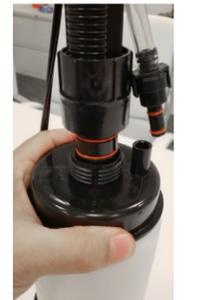
7. Rotate the Bottle back and forth to align the flat section of the Stem to the flat section on the Bottle.
