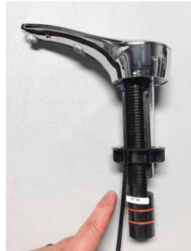
3. Place the Wave Washer on top of the Mounting Nut. Install Mounting Nut on Stem and thread upwards. (Minimum 2-1/4" (55mm) diameter clearance needed below mounting nut).
