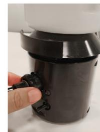
11. Thread Fiber Optic Nut onto Connector Port and hand snug only. Do not over-tighten.
