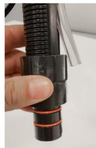
4. Thread the Stem Locking Nut onto the Stem. The ribs on the Nut are to be towards the top. Once it goes past the two red o-rings, the nut will automatically stop threading.
