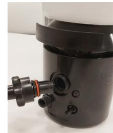
10. Insert Fiber Optic Connector Tip into Bottom Housing. Keyed feature on Connector Tip ensures Fiber Optic Cables are always located correctly.
