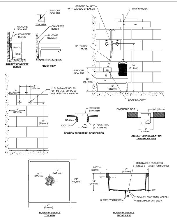
**Installation Note:** QIC32 Quick Drain Connector for 2" pipe or QIC3SN Quick Drain Connector for cast iron soil pipe must be ordered separately. **IMPORTANT:** Roughing-in dimensions may vary 1/2" and are subject to change or cancellation without prior notice.
