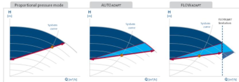
Proportional pressure mode is used in circulating systems. The pump continuously adapts its performance to the varying flow demand.
