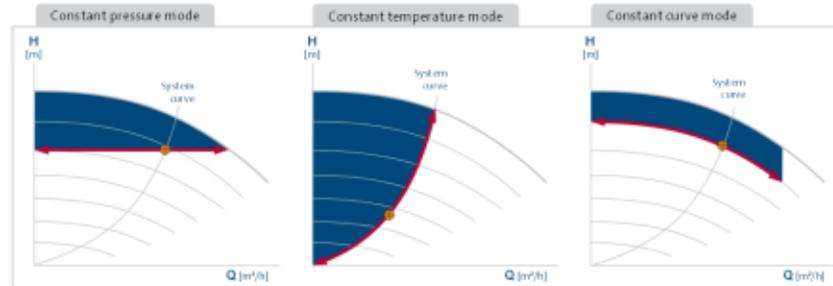
Constant pressure mode is suited for variable flow systems with very low pipe pressure losses, and in open systems where pipe pressure loss is subordinate to static head.
